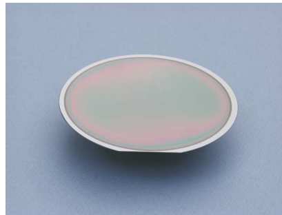
The colored fringes indicate a \pm 5\% uniformity of the deposited diamond film on this 100mm wafer.
