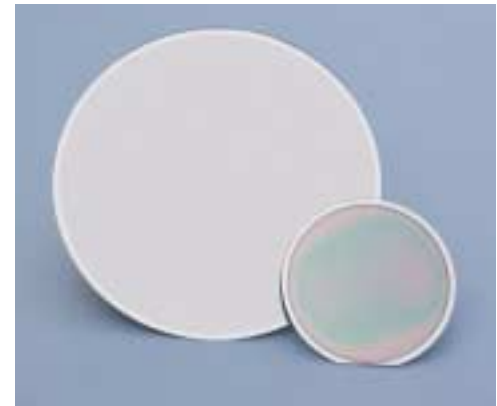
200mm and 100mm diamond coated silicon wafers. The colored fringes indicate a \pm 5\% uniformity of the deposited diamond film on this 100mm wafer.
